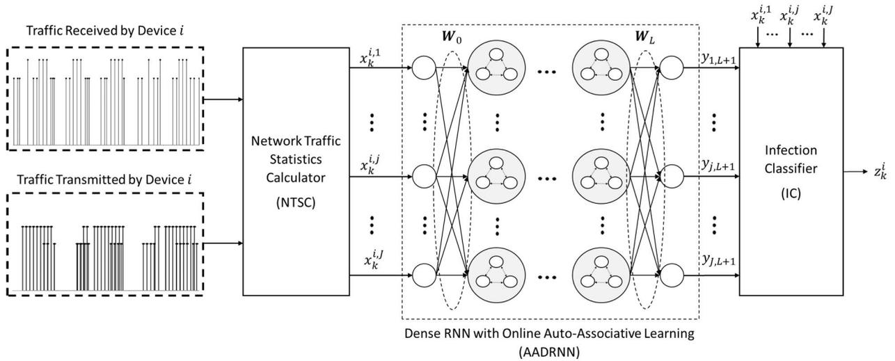
**FIGURE 2.** Compromised device identification system (CDIS) whose inputs are received and transmitted traffic flows of IoT device  $i$ , output is infection decision, and architecture consists of Network Traffic Statistics Calculator (NTSC), AADRNN and Infection Classifier (IC) modules.
