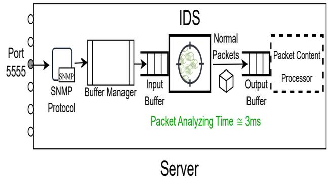
Fig. 2. Internal software architecture of the Server, containing a SNMP network protocol manager, an AD system [30] that identifies attack packets, and software for processing the incoming packet contents.
