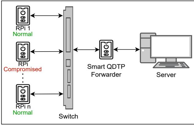
Fig. 6. The figure shows the modified system architecture where a Smart QDTP Forwarder (SQF) constantly acts as a traffic shaping interface between the Ethernet LAN and the Server. The effect of the SQF is to eliminate the paralyzing effect of the packet flood at the Server, buffering packets within the SQF and forwarding in a manner which allows the Server to conduct its AD processing and other work in a timely fashion.
