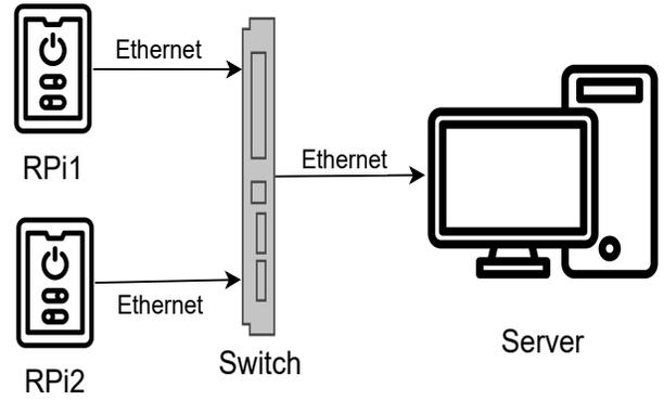
Fig. 1. The test-bed composed of an Ethernet network with Raspberry Pi machines that generate normal traffic, as well as possible traffic. An IoT Server receives the IoT traffic via the same network.
