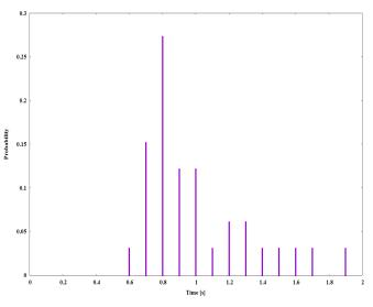
Fig. 13. Distribution of Routing Engine Reaction Time to a sudden substantial change in the Trust Metric T(.,.).
