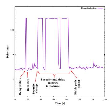
Fig. 14. System reactions to changes in delay and security. Note that the x-axis describes the course of real events in seconds, while the y-axis plots the reaction times of the system as a whole, in milliseconds, to the events that occur along the x-axis.
