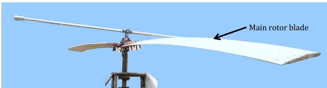
**Figure 4: Realized and mounted main rotor blades.**
